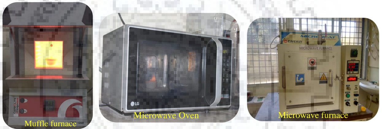
Figure 3.14 The equipment used for carbothermal reduction
