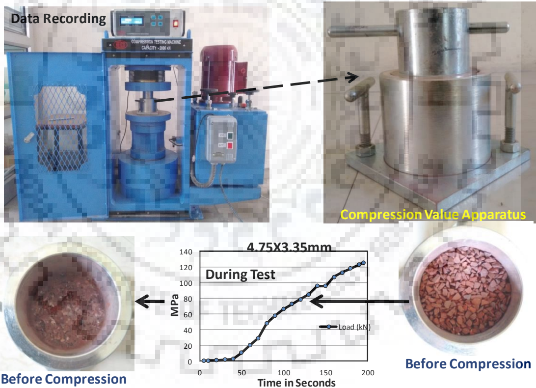
Figure 3.7 Compression test setup
