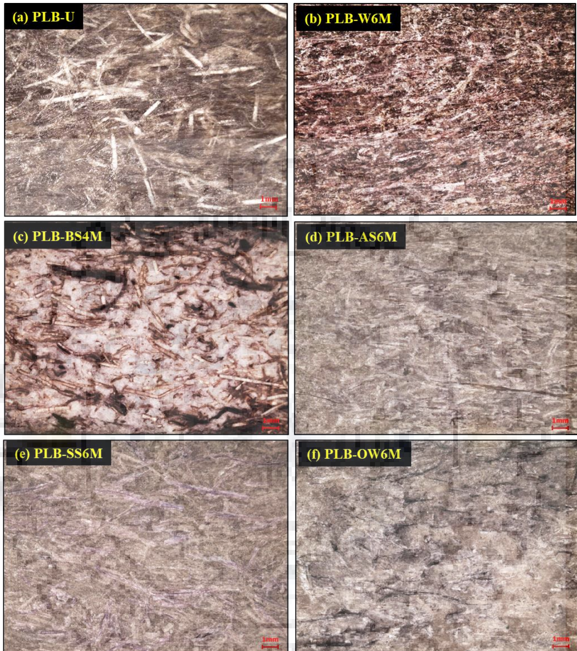
Fig. 6. 13 SM images of surface of PLB composites before and after 6 months (4 months in case of basic solution) of exposure
