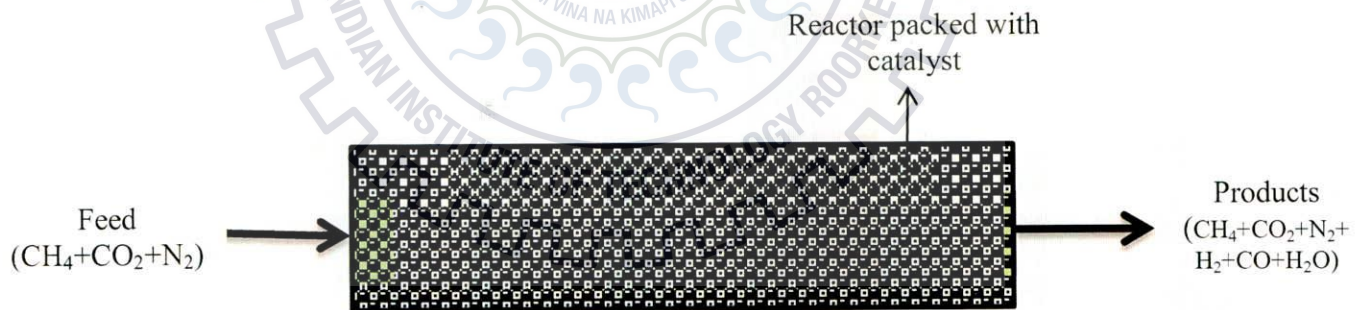
Fig 3.2: Schematic Representation of Fixed Bed Reactor.
