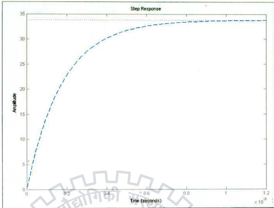
Figure 4.3 Step response of the converter without controller
