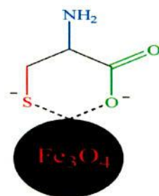
Figure 2: Shows the interaction between magnetite and cysteine molecule
