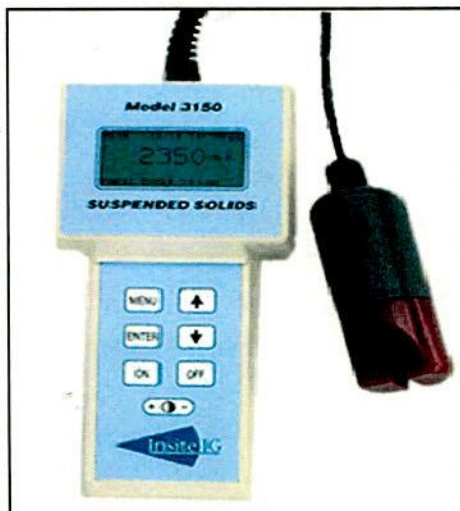
Fig. 3.10: Suspended Solids Analyzer
