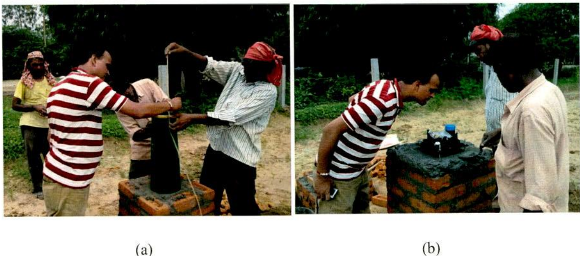
Fig. 4.12 Setup of (a) Ordinary Rain Gauge and (b) Self – Recording Rain Gauge
