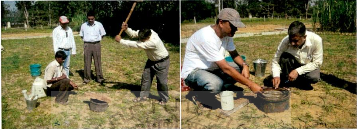
Fig. 4.16a Double Ring Infiltrimeter Test in each experimental plot.
