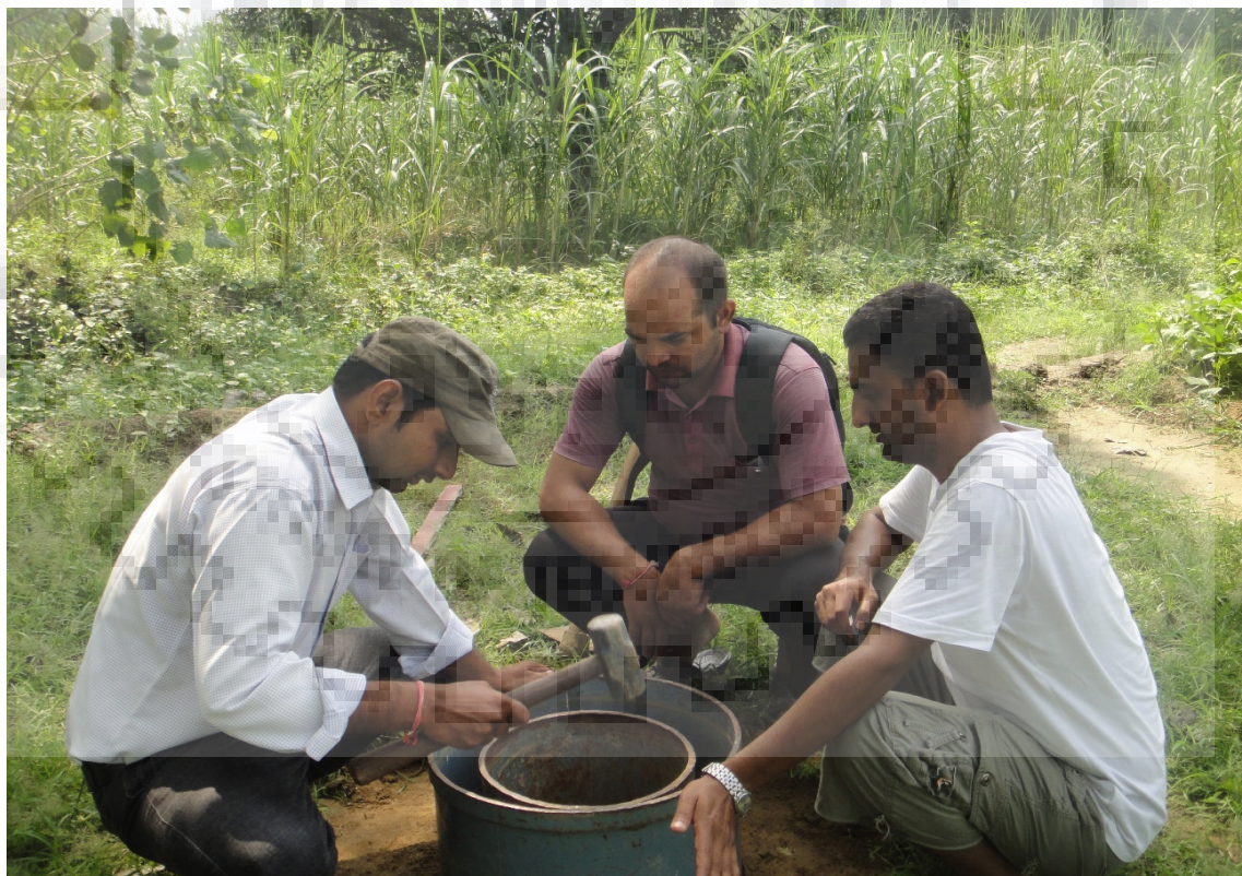
Figure 3.7a Installation of double ring infiltrometer in the fallow plot
