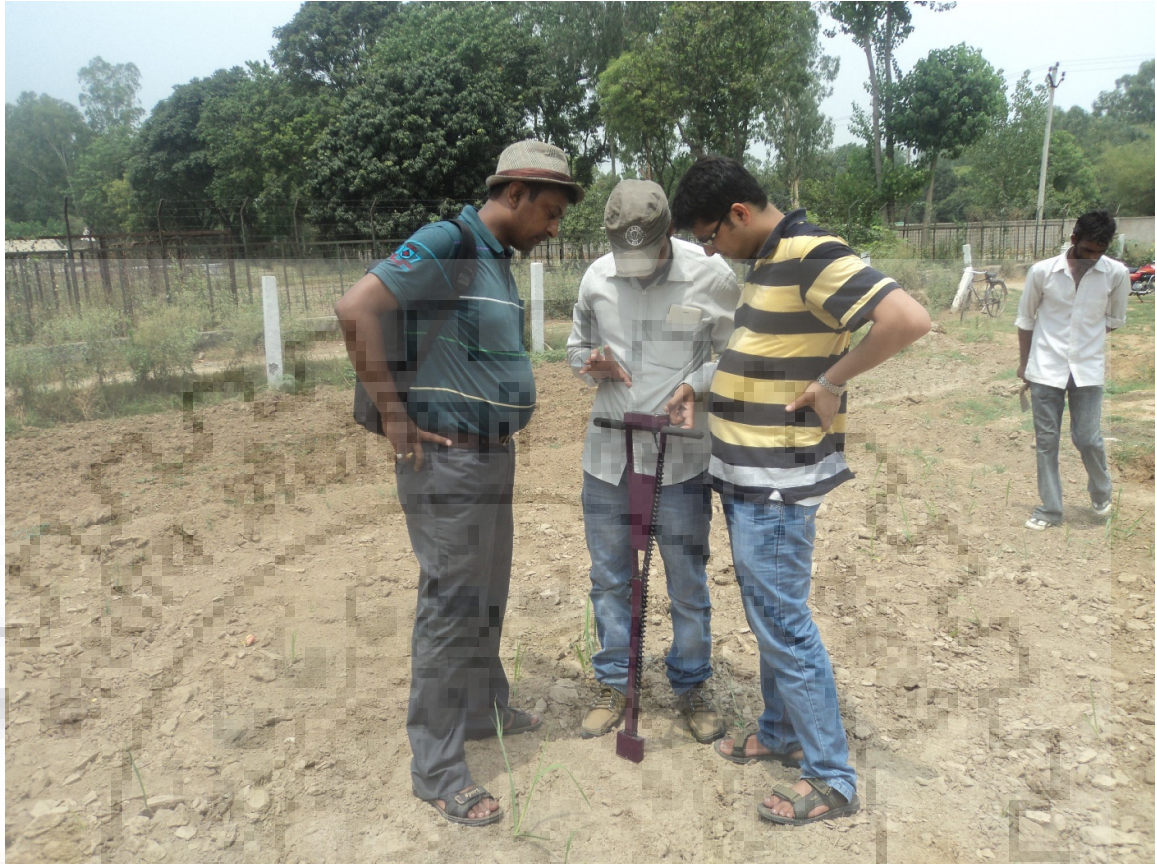
Figure 3.8 Measurement of soil moisture in sugarcane plot at middle side
