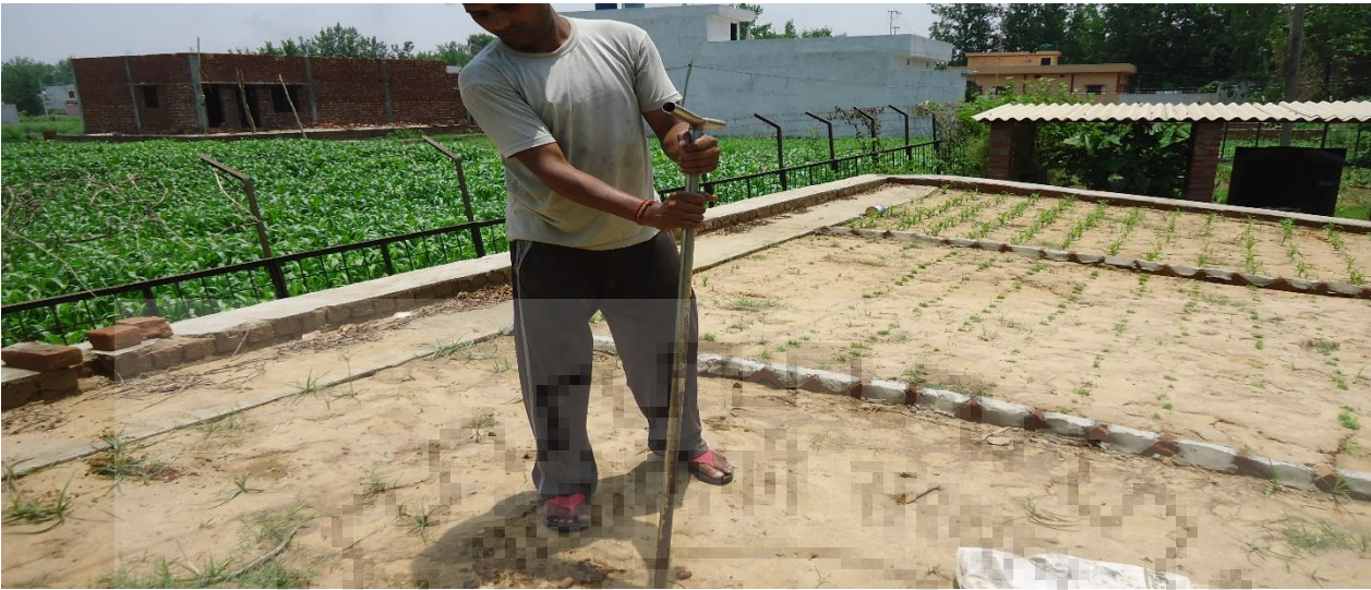
Soil sampling for grain size analysis of soil
