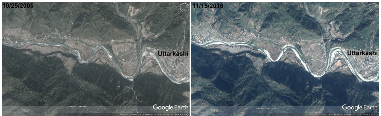
Figure 4.10. Google Earth images over a segment of Bhagirathi River showing increase in deposition along upstream part of the channel after construction of Tehri dam. The Tehri dam, present day local base level of Bhagirathi river have reduced the channel slope of the river. As a result deposition has increased along the upstream part (from the reservoir) of the channel.
