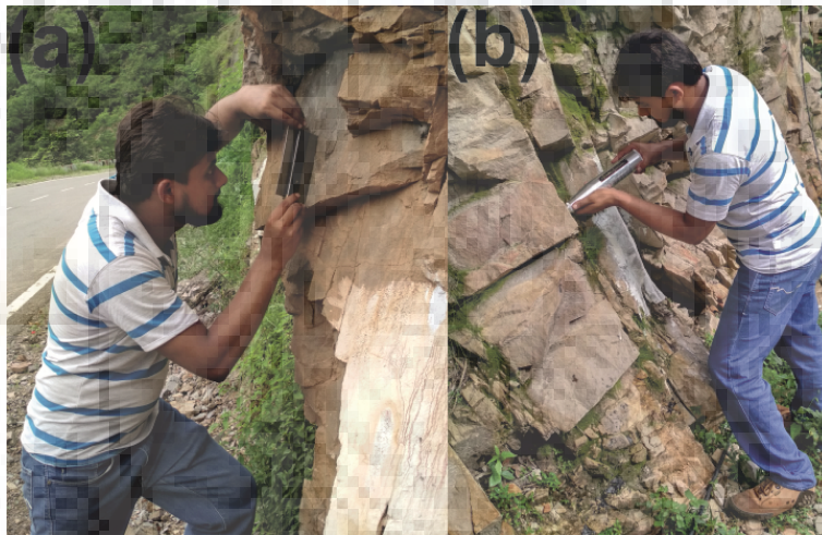
Figure 3.24: Measurement of geotechnical parameters during field survey (a) Roughness profile of joint wall by using Barton comb (b) Schmidt hammer hardness of jointed surface
