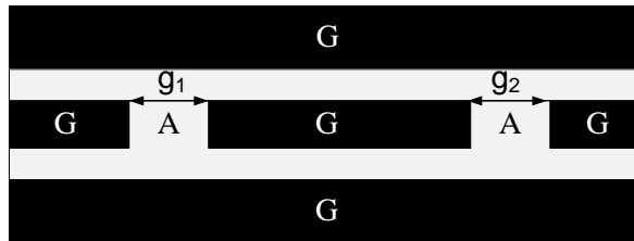
Fig. 3.2.1.2 Design of resonator. Here, G denotes graphene and A stands for air.
