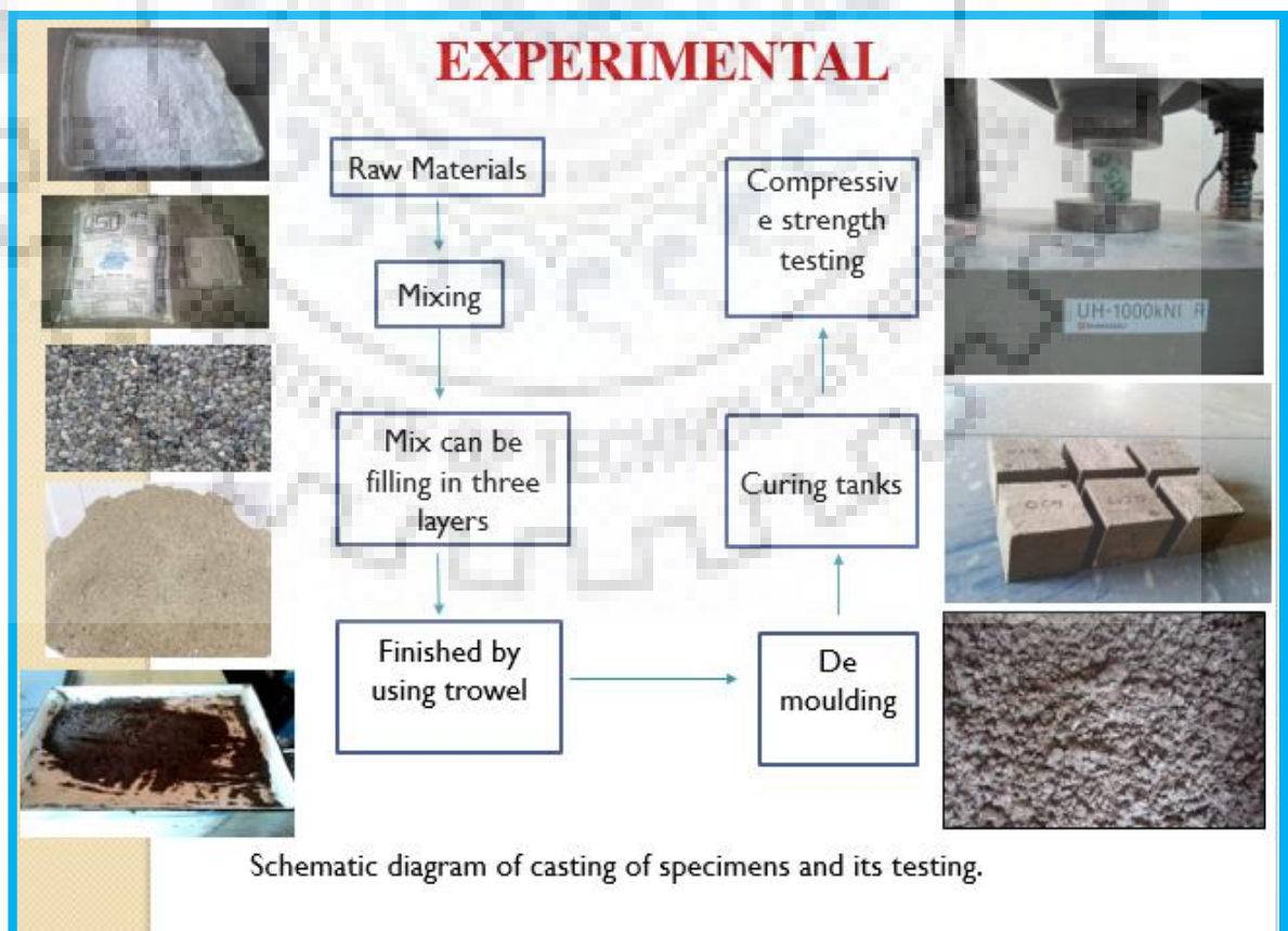
Fig. 3.4: Schematic diagram of casting and testing of specimen
