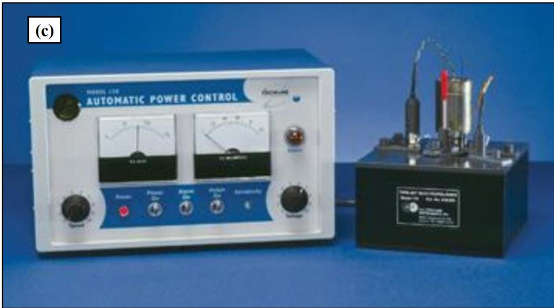
Fig. 3.14: Photograph of the TEM sample preparation unit (a) Gatan punching tool (Model: 656 punch), (b) Dimple grinder (Model: Fischione 200) (c) Twin jet electropolisher.
