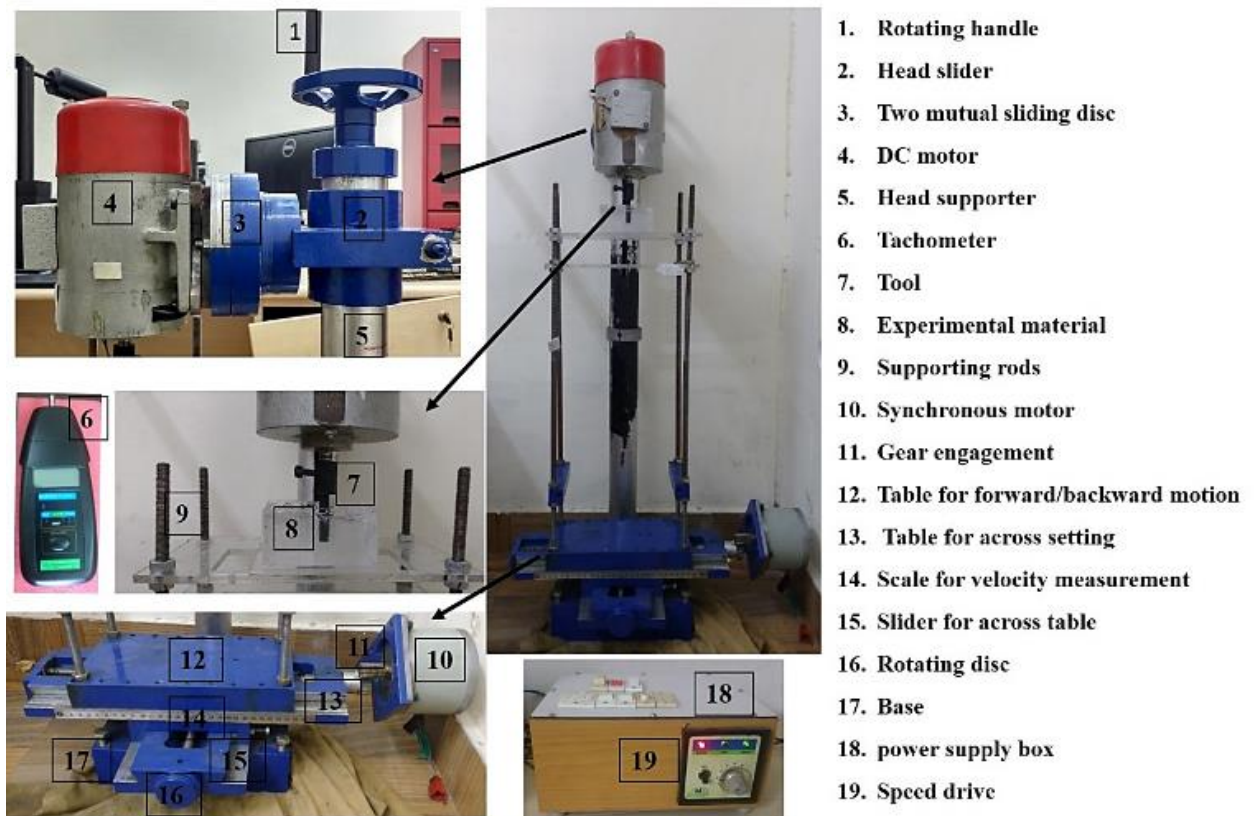
Fig. 4.10: FSW machine model for PIV application.
