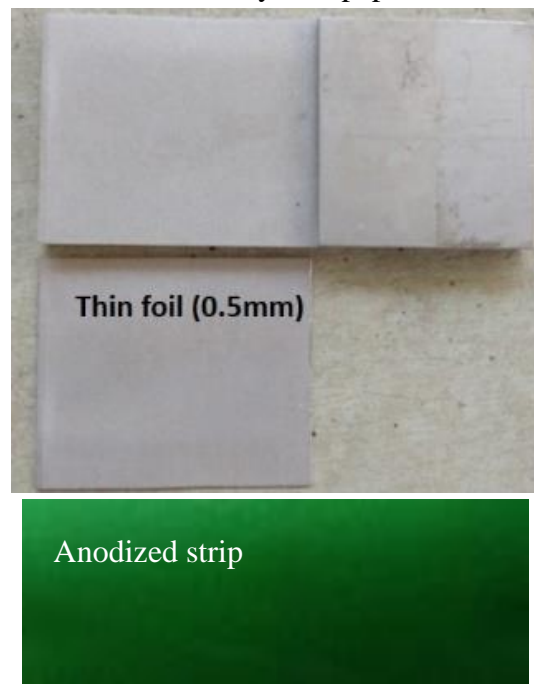
Fig. 4.1: Tracer preparation from workpiece material.
