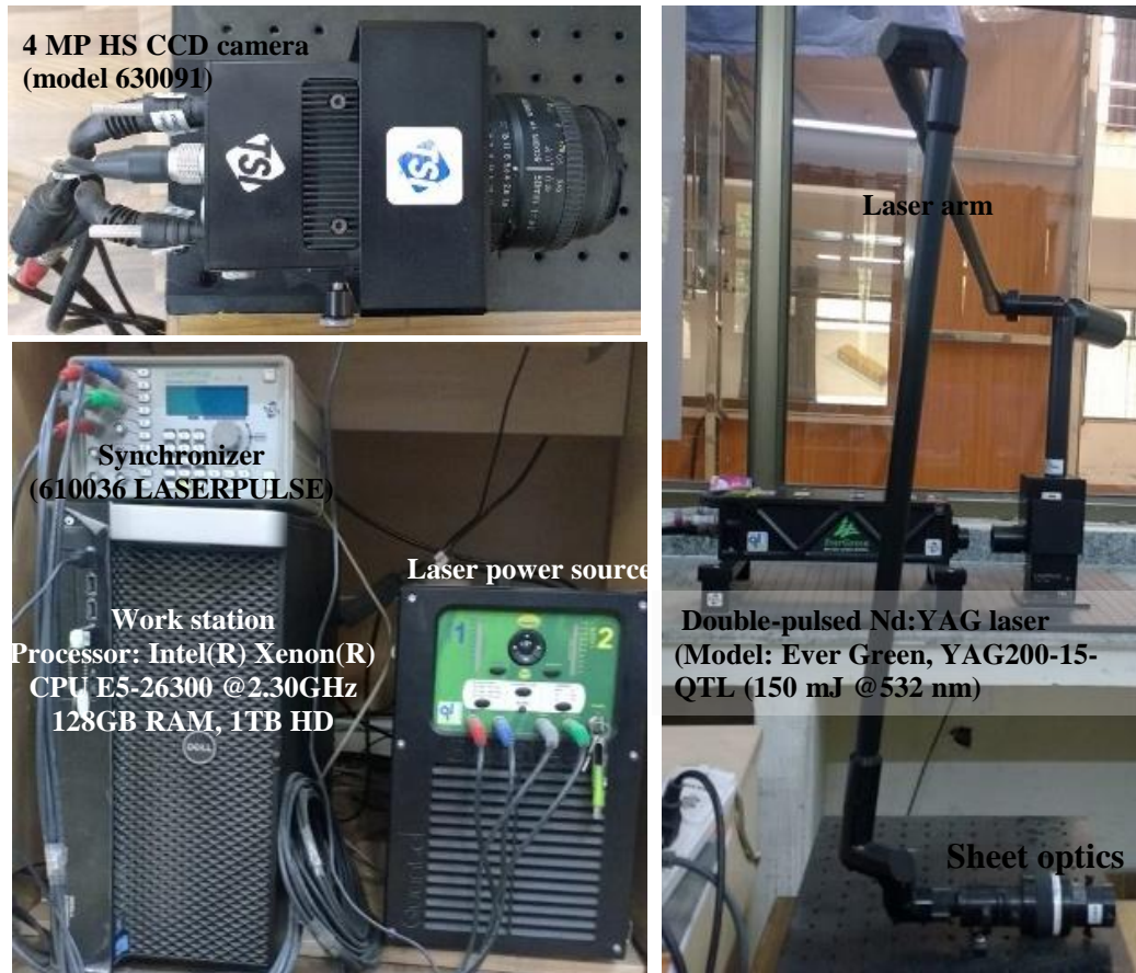
Fig. 4.11: PIV system parts: CCD camera, synchronizer, workstation, laser power source, laser head, laser arm and light sheet optics.
