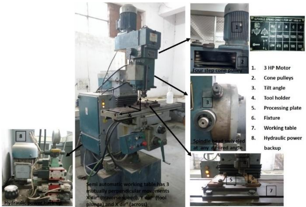
Fig. 4.3: FSW machine setup.
