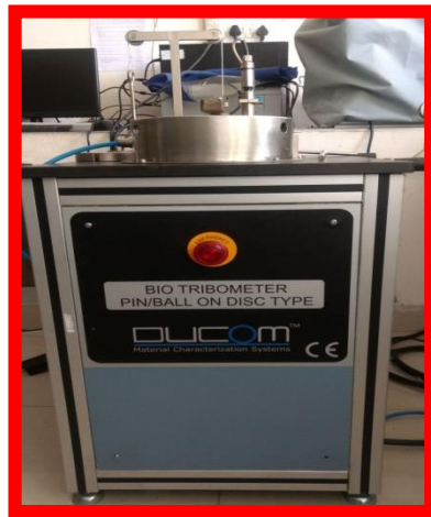
Fig. 3.11 Digital image of the ball-on-disk tribometer to perform continuous sliding wear test
