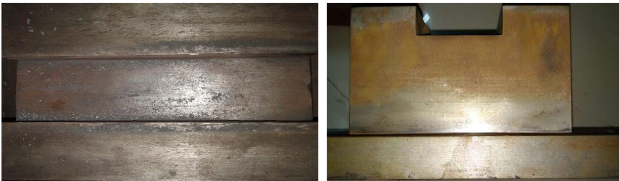
Figure 4.4: A channel die of dimension 220(l) × 75(w) × 25(h) mm 3 .
