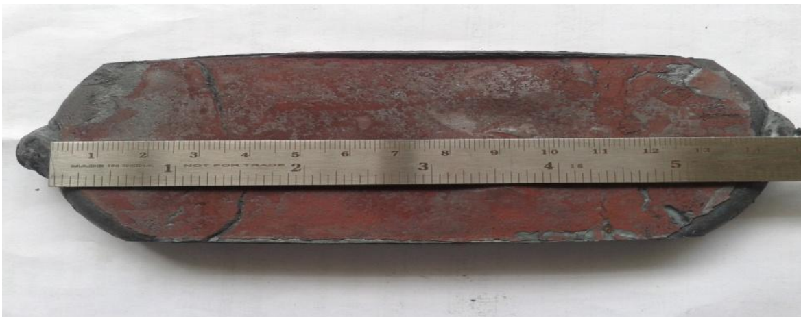
Figure 4.8: Forged slab after removing both gas flow pipes.
