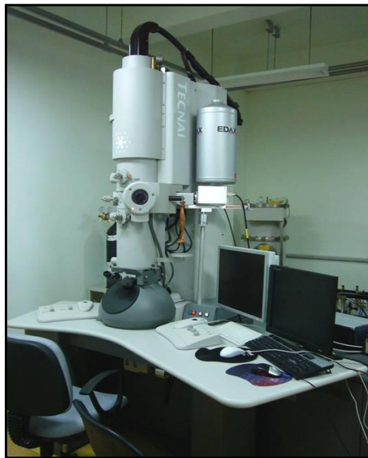
Fig. 3.8c: Photograph of the TEM unit (FEI Tecnai-20 G2S-TEM).
