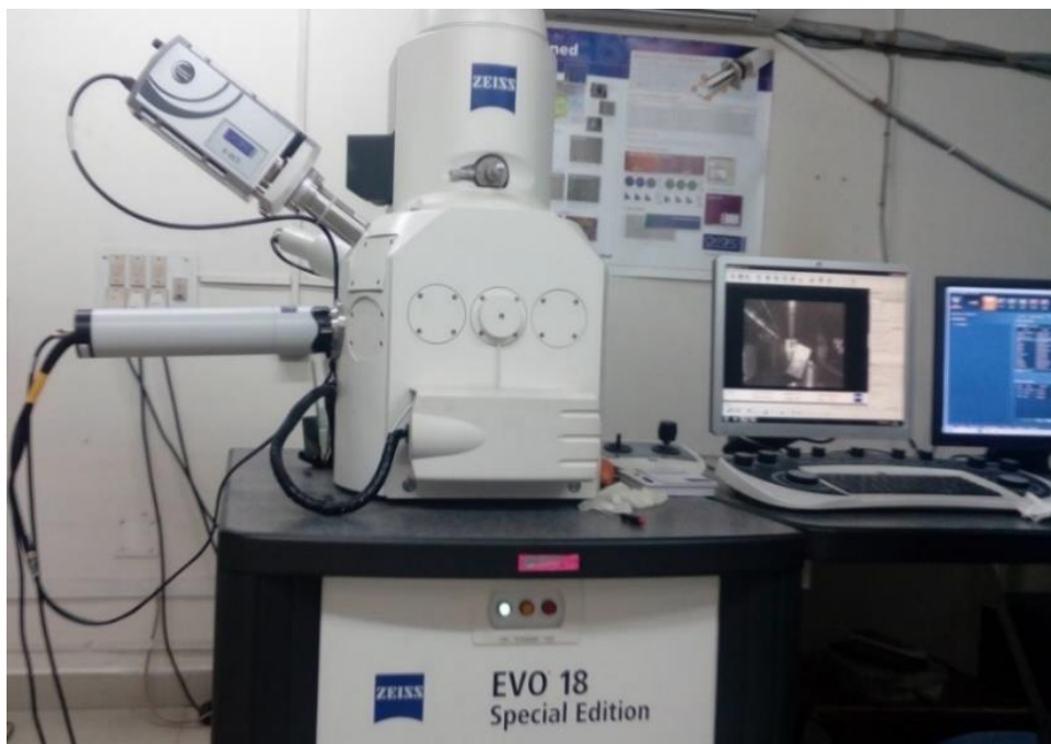
Figure 3. 8 ZEISS EVO 18 Special Edition scanning electron microscope used for characterization of in-situ aluminide reinforced aluminium alloy composites.
