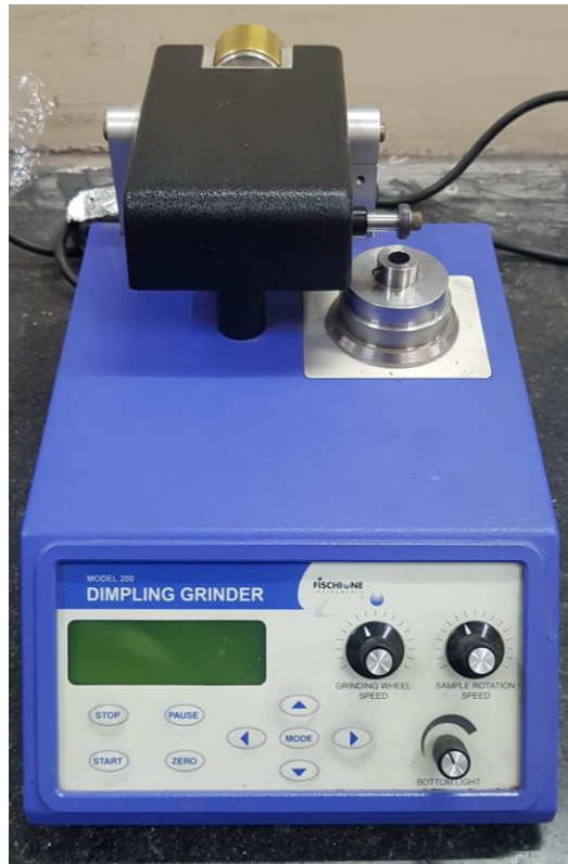
Figure 3. 5 Dimple grinder for creating dimple at the centre of the thin slice
