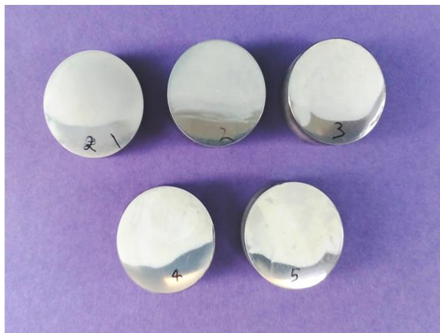
Fig. 4.44 Spark plasma sintered nano composite samples starting from top left.
