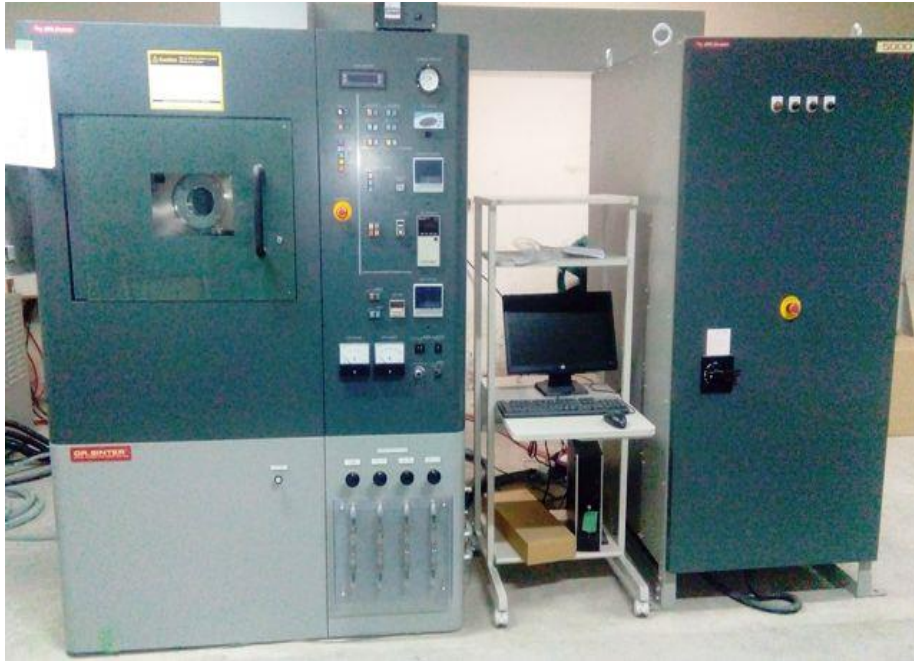
Fig. 3.8 SPS equipment used in the present study.
