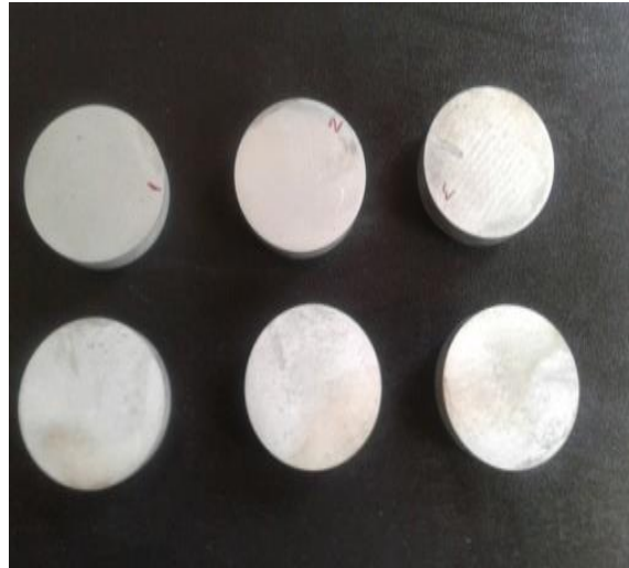
Fig. 4.20 SPSed composite samples reinforced with varying amounts of yttrium.
