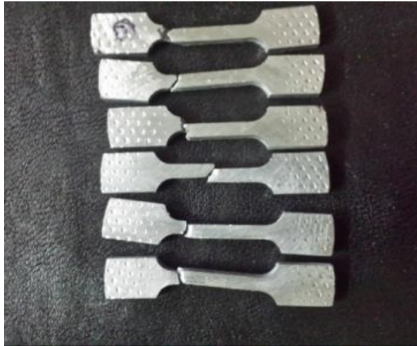
Fig. 4.34. Fractured tensile specimens reinforced with varying wt% of yttrium (starting from minimum yttrium at the top to maximum yttrium at the bottom).
