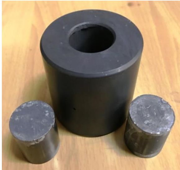
Fig. 3.10 Die and punches used to develop the composite samples.
