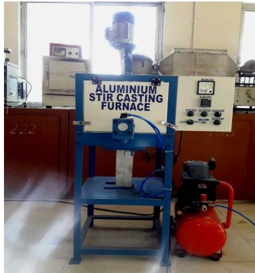
Fig. 3.6 Aluminium stir casting furnace set-up used in the present investigation.
