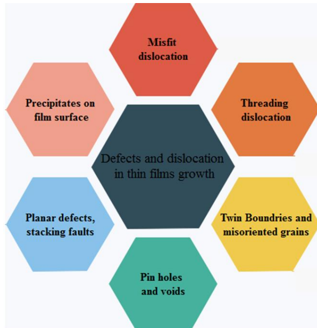
Figure 1.3. Schematic diagram showing defects induced in thin film during synthesis.
