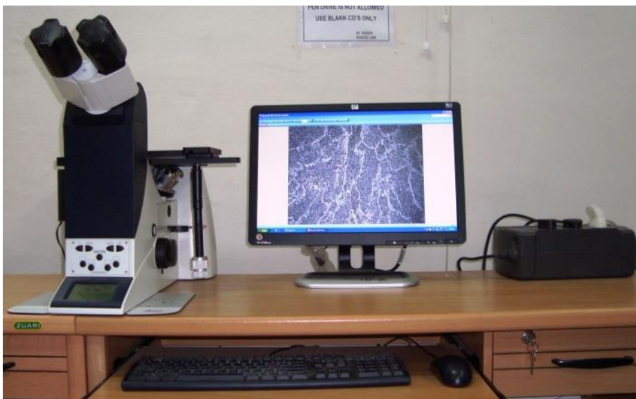
Fig. 4.9 Photograph of the Leica optical microscope used for recording microstructure.
