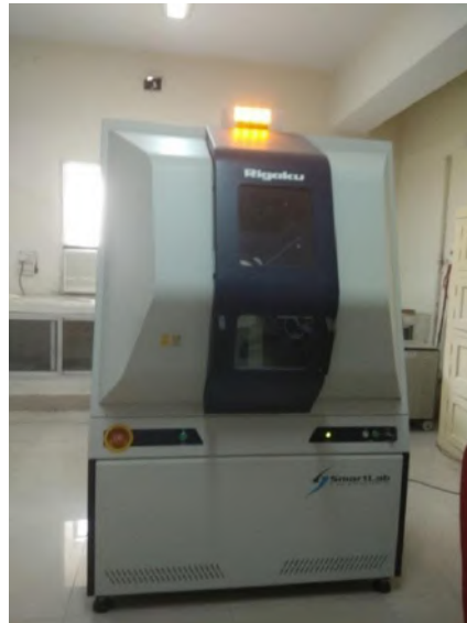
Fig. 4.11 Photograph of the X-ray Diffractometer used for analysis of phases.
