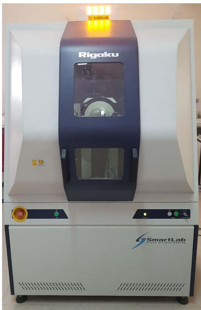
Figure 3.11. XRD (Rigaku SmartLab) used for characterization of binary aluminium alloys.
