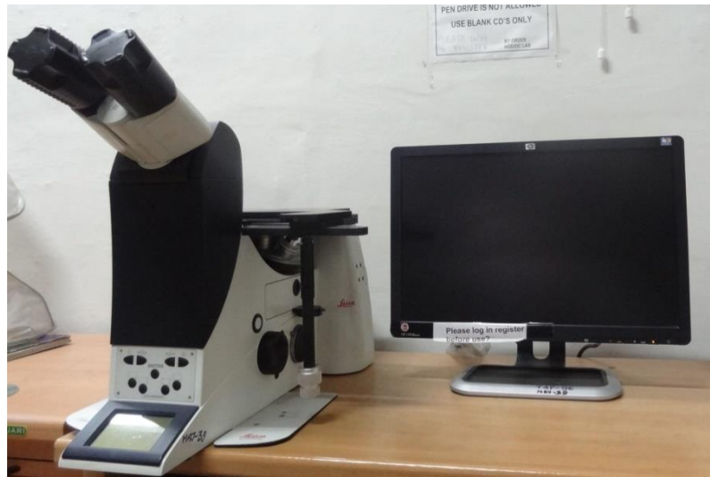
Figure 3.8. Leica (DMI5000 M) optical microscope was used for optical microscopy.
