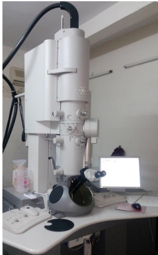
Figure 3.10. Transmission electron microscope (FEI Netherlands) used for characterization of aluminium alloy composites.
