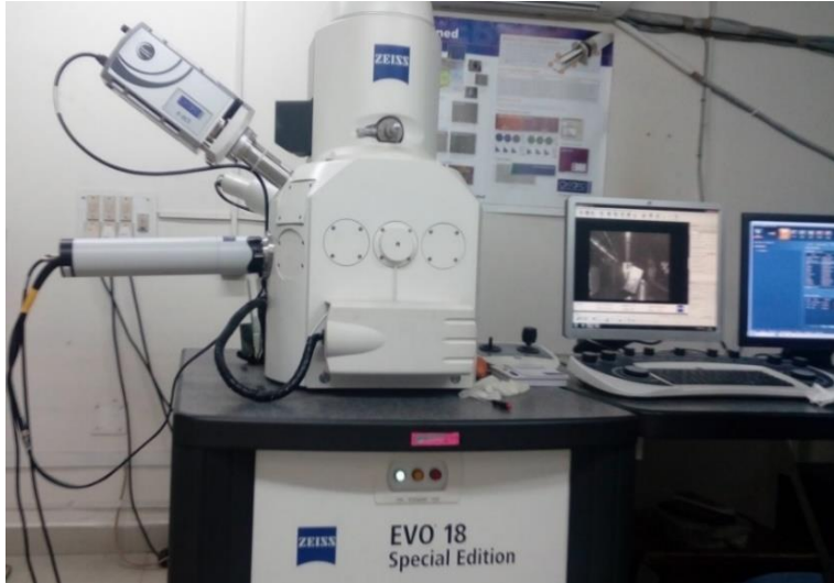
Figure 3.9. ZEISS EVO 18 Special Edition scanning electron microscope used for characterization of binary aluminium alloys and aluminium alloy composites.
