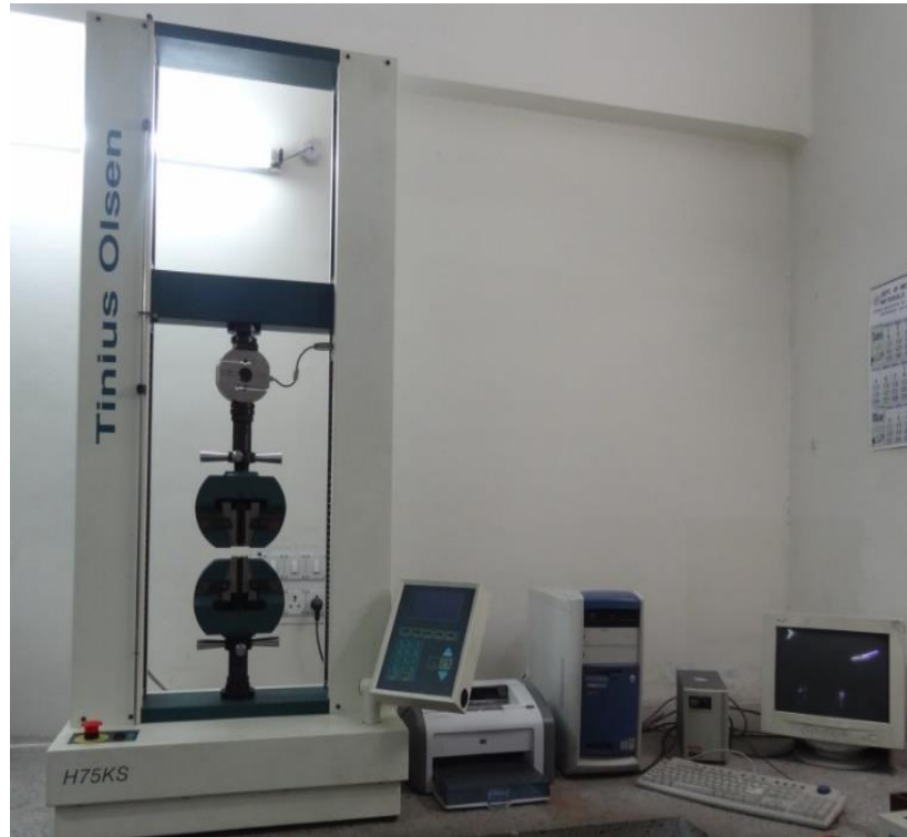
Figure 3.13. H25 K-S Tinus Olsen tensile testing machine used for the tensile testing of aluminium alloys and aluminium alloy composites.
