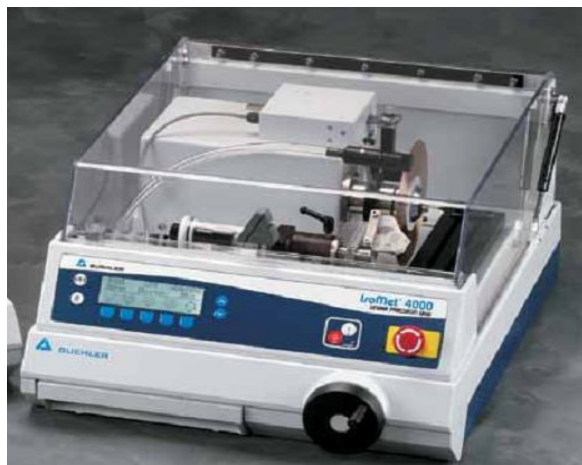
Figure 3.7. Diamond cutter IsoMet 4000 for cutting the sample.
