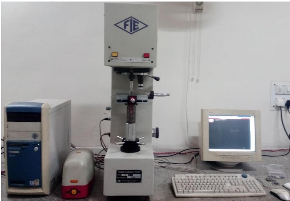
Figure 3.12. Vickers hardness testing machine (FIE Model VM 50) used for the measuring the hardness of aluminium alloys and aluminium alloy composites.
