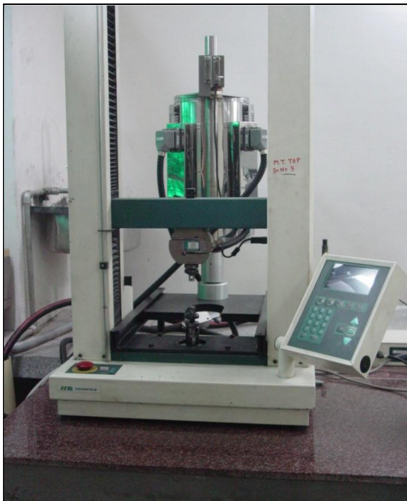
Fig. 3.5.2.3. H-25K tensile testing machine (Capacity 25 kN)
