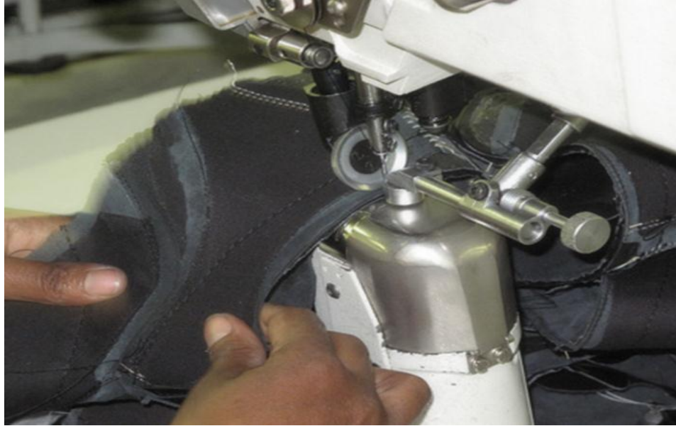
Figure 2.8 Leather stitching operation: Taken from stitching department of Anbesa Shoe company (Phot credit: Gebeyehu (2014))
