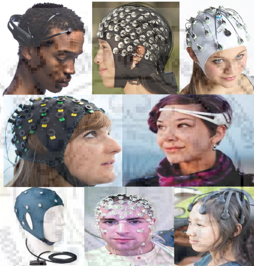
Figure 6.2: Various EEG devices that have been used in research. All devices has varying number of electrodes from 5 to 128.
