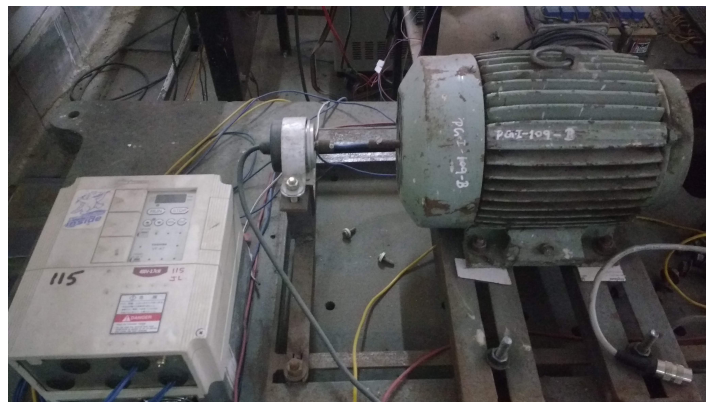
Fig. 2.7: Induction motor with high-performance inverter operating as a prime mover.
