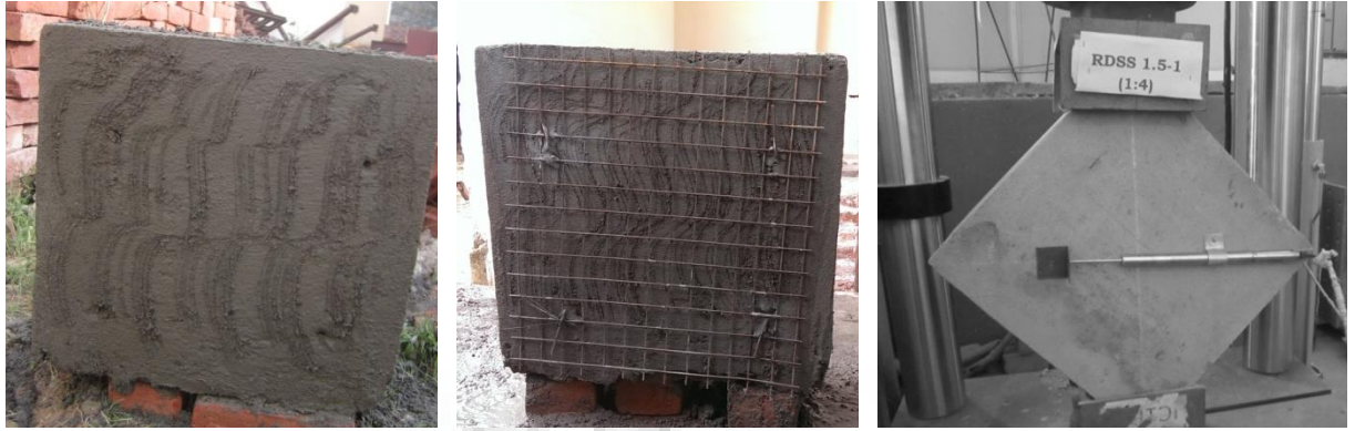
Figure 2. 3 : Stages of strengthening unreinforced specimen with WWM
