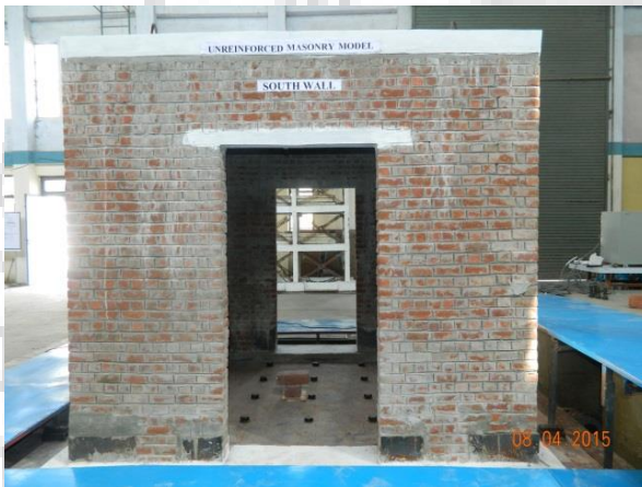
Figure 4.8 : Front facing URM building model
