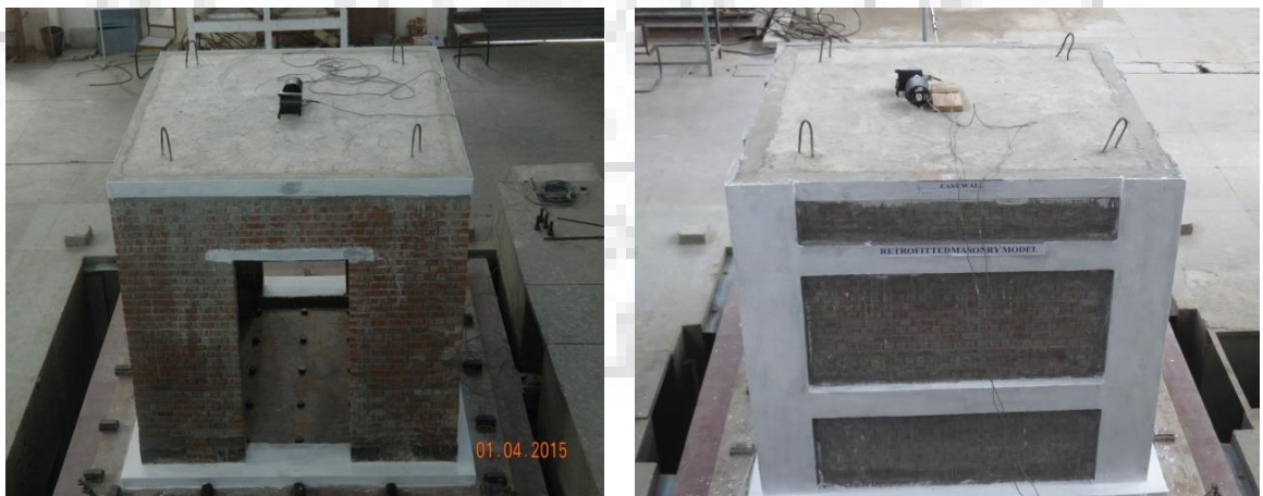
Figure 4. 14 : Free vibration setup for URM model and RM model
