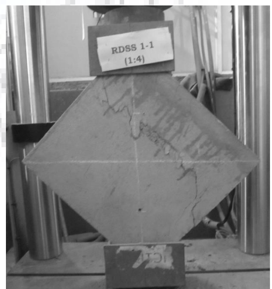
Figure 2. 6 : (a)-(b) High strength mortar retrofitted panel with 1 inch , 1.5 inch and 2 inch spacing WWM (contd.)
