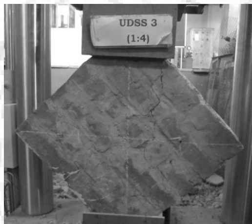
Figure 2. 5 : URM specimen after testing
