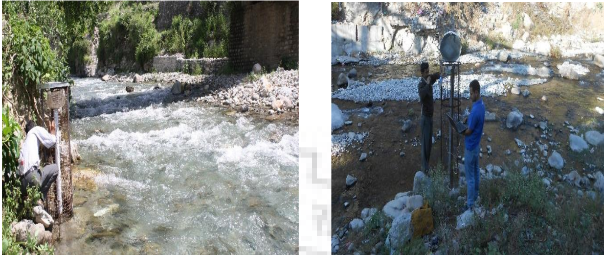
Figure 4.5 a) Medium flow condition and AWLS in PVC pipe b) Data downloading from Odyssey data logger
