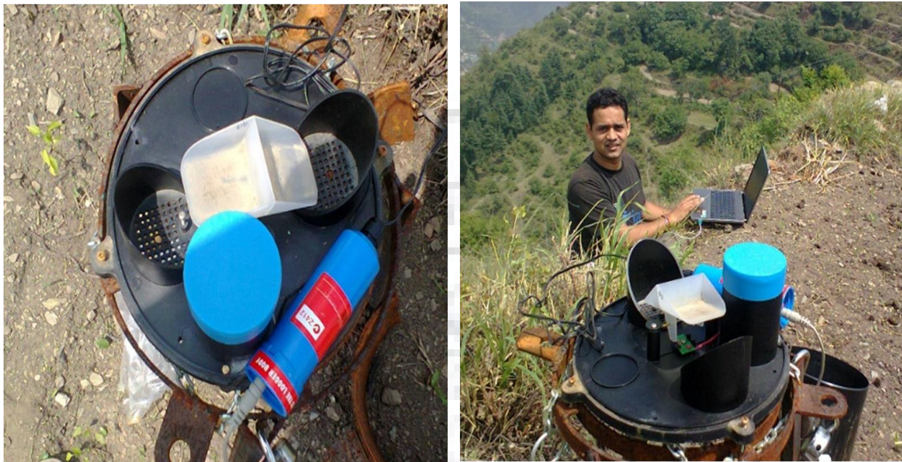
Figure 4.2: a) Tipping bucket b) Data downloading from tipping bucket
