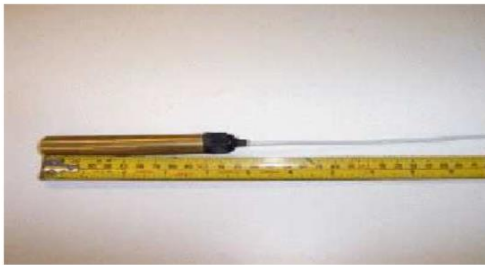
Figure 4.6 Calibration of water level logger
