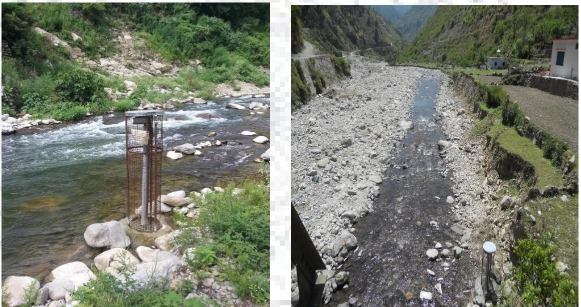
Figure 5.2: Location of Gauging station with deployed water logger and caging to protect the logger
