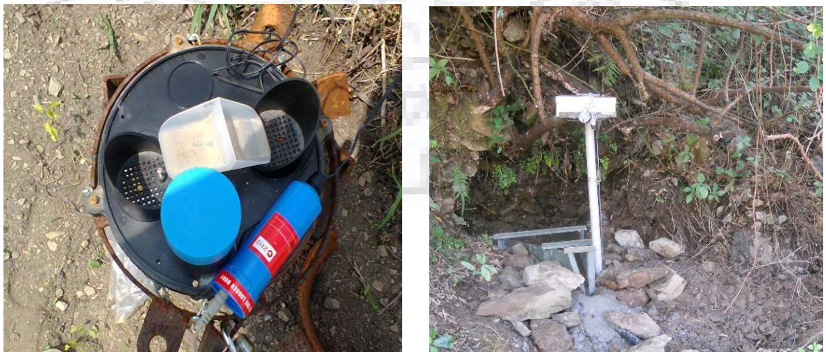
Figure 6.4: Field instrumentation (a) Tipping Bucket (b) HS Flume with data logger
