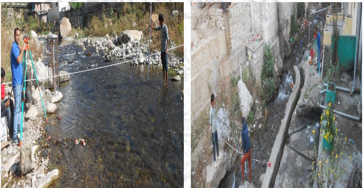
Figure 5.4: Cross section plotting and discharge measurement using current meter
