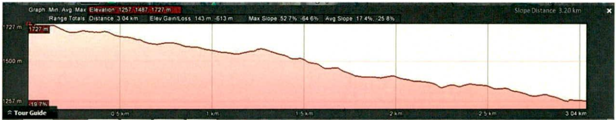
Figure 19: The Slope profile of Escape Route 2
