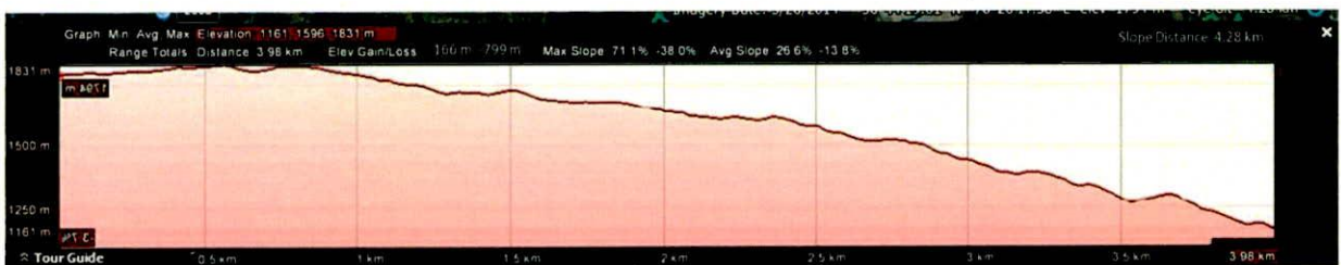
Figure 18: The Slope profile of Escape Route 1
