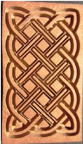
Figure 6.43 Engraving in geometrical pattern by using CNC wood engraving machine
