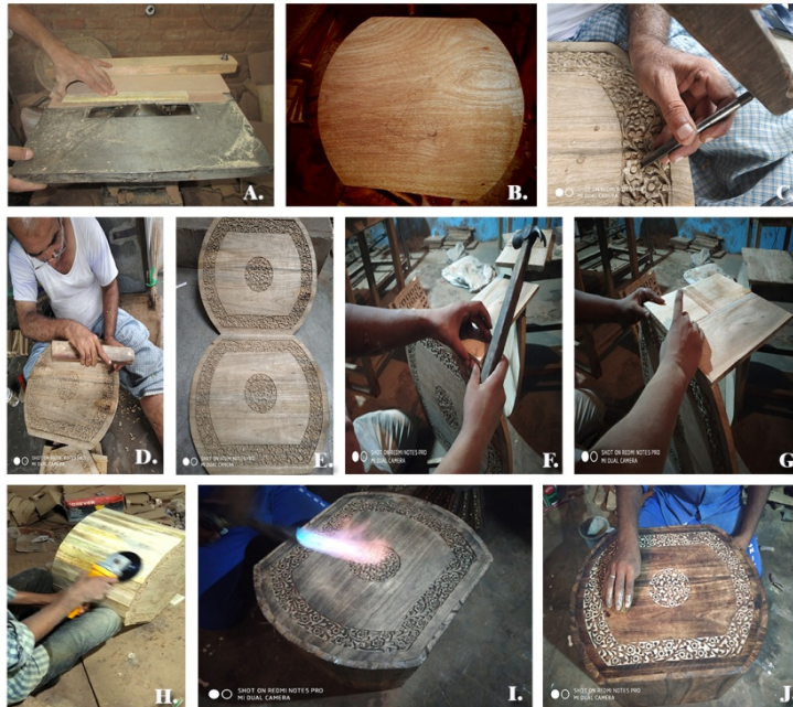
Figure 6.7 Manufacturing process of stool cum side table
