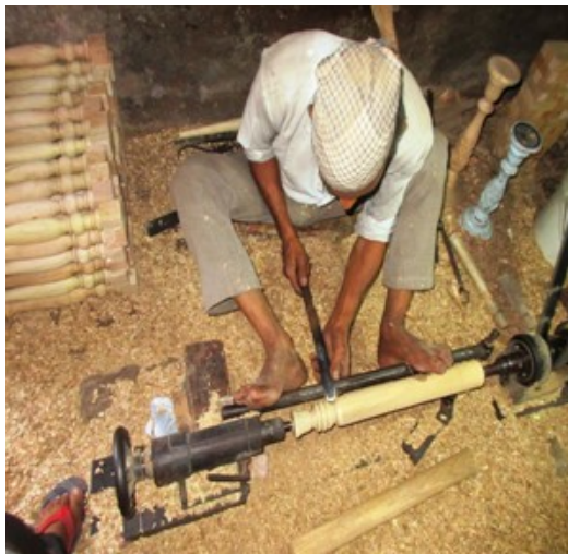
Figure: 4.40 Artisan working with lathe machine
