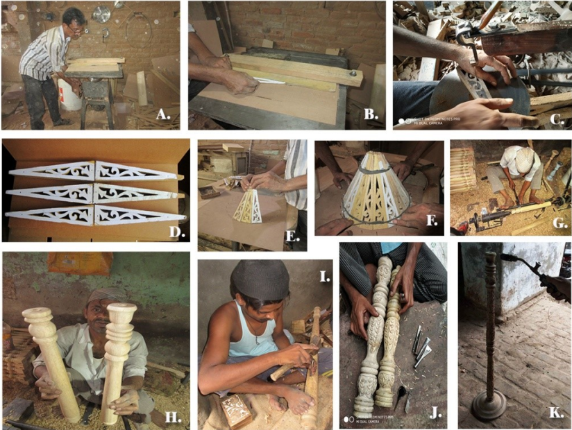
Figure 6.4 Manufacturing process of wooden lamp shade
