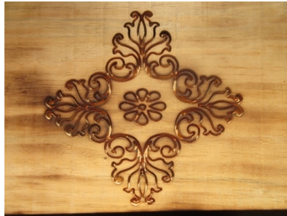
Figure 6.43 Engraving in geometrical pattern by using CNC wood engraving machine
