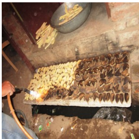
Figure 4.29 Burner flames being used for antique look
