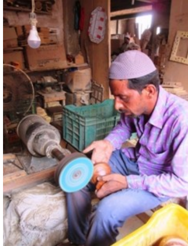
Figure 4.42 Sanding being done by the artisan
