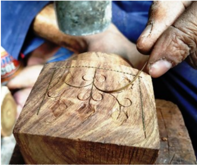
Figure 4.36 Inlay work of brass wire
