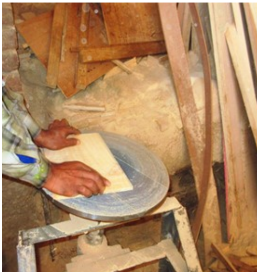
Figure 4.21 Artisan using the planer
