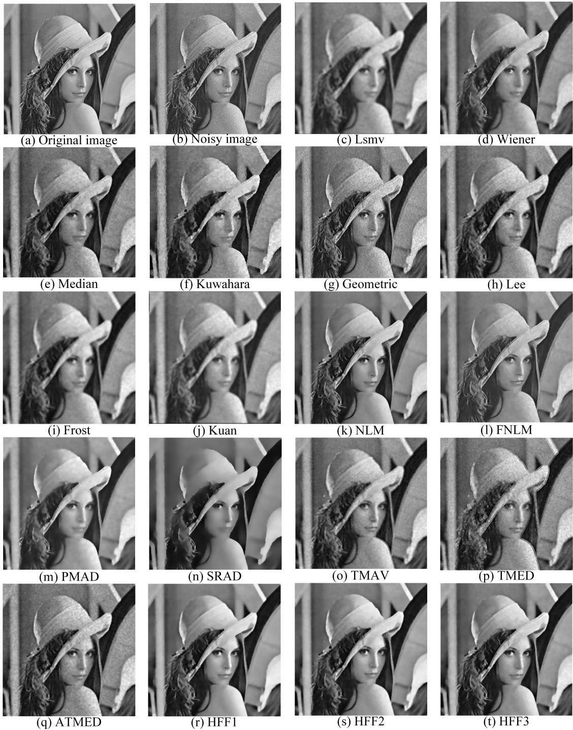
Fig. 3.3: Visual quality comparison of denoised Lena image for noise level equal to 0.01 using different filters
