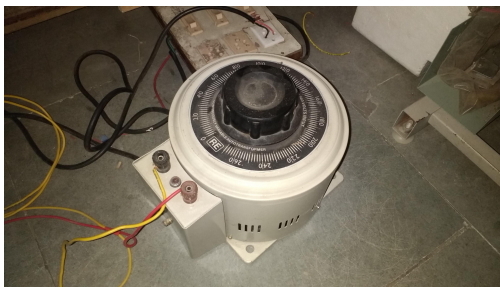
(c) Single-phase auto transformer
