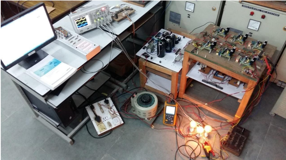
Fig. 1: Front view of the experimental set-up and host computer running D-SPACE.
