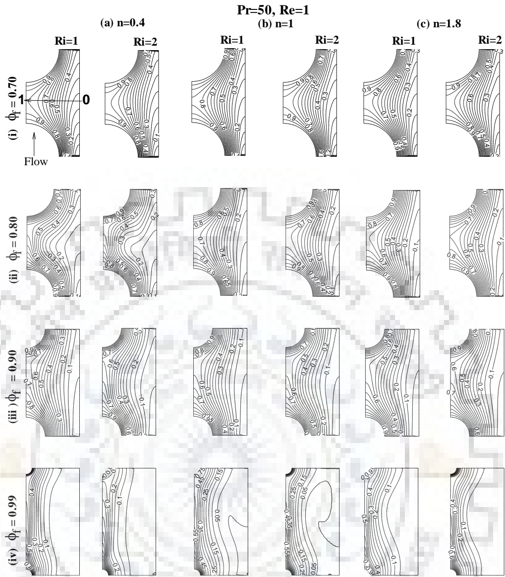
Figure 9.10: Dependence of normalized isotherm patterns over the power-law index ( n = 0.4, 1, 1.8 ), fluid volume fractions ( \phi_f = 0.70, 0.80, 0.90, 0.99 ) and Richardson number ( Ri = 1 and 2 ) at a fixed values of Prandtl number ( Pr = 50 ) and Reynolds number ( Re = 1 )
