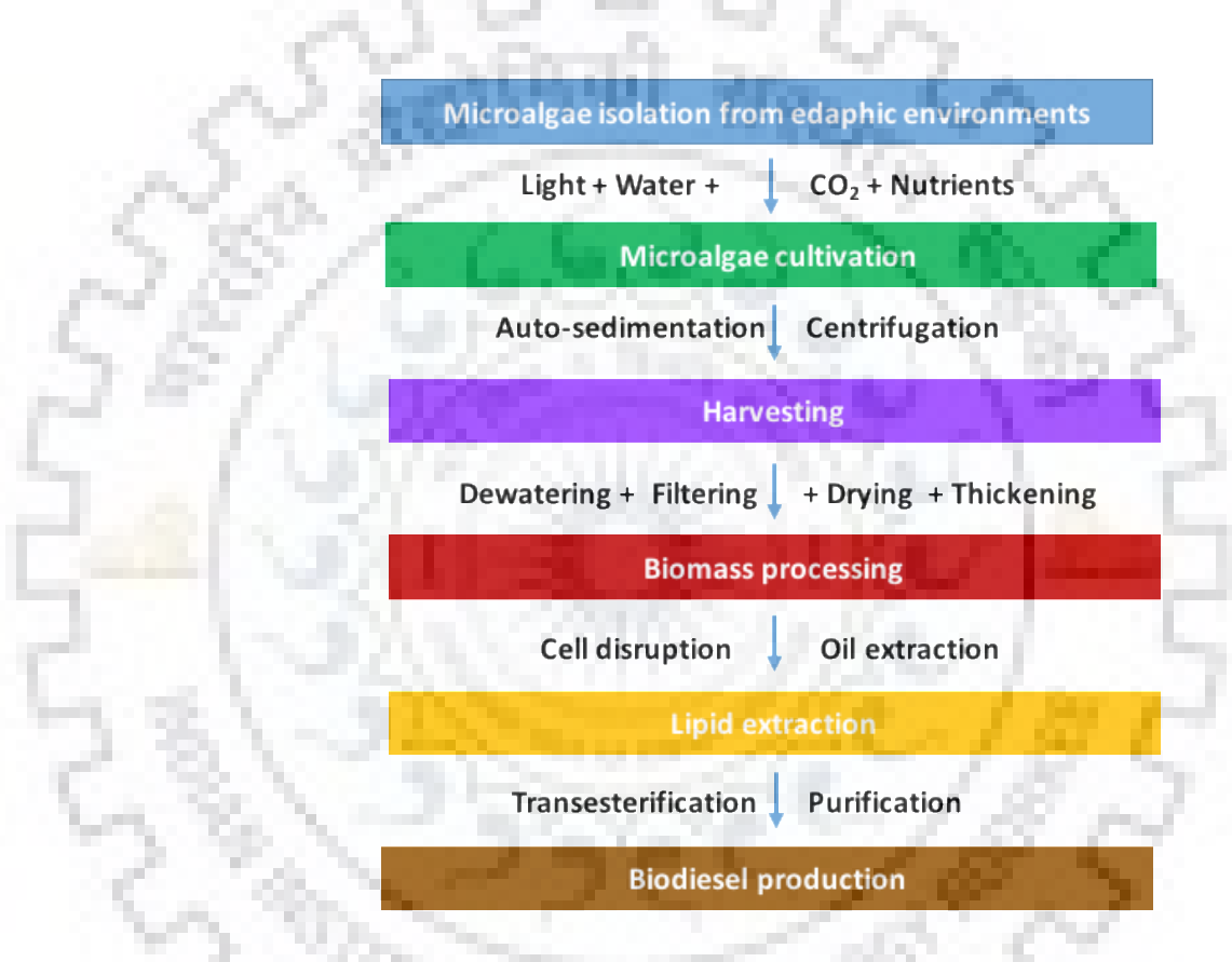
Fig. 1.3: Flow chart of biodiesel production from microalgae.
