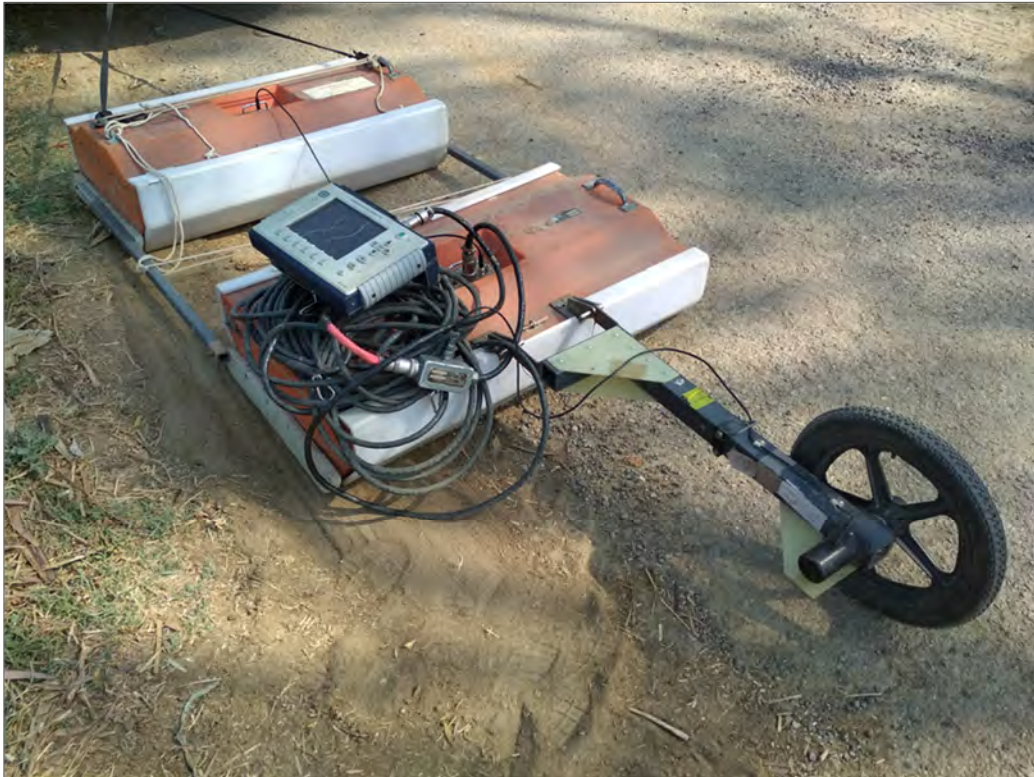
Figure 6.4 Ground penetrating radar (GPR) setup with survey, shielded antennae, control unit and fibre cables for survey in distance mode.
