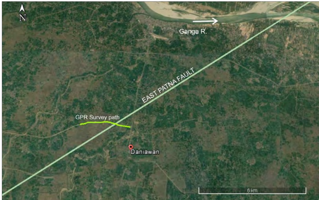
Figure 6.2 Location of ground penetrating radar (GPR) survey carried out across East Patna Fault (EPF) near Daniawan village in Patna, Bihar. The base image is obtained from Google Earth.
