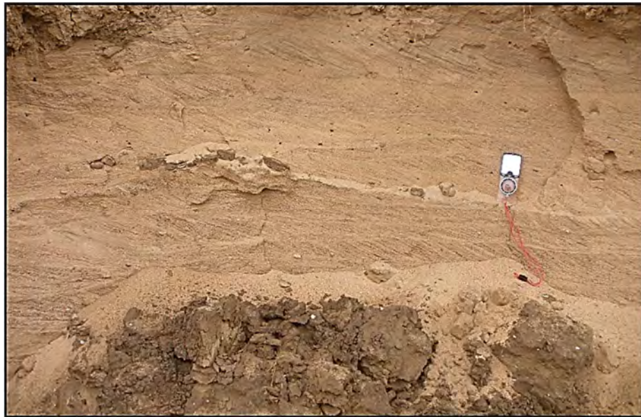
Figure 3.9 The cross-stratification structures are shown by the sand beds deposition indicating fluvial environment. Topset and foreset dipping 3° and 22° respectively towards NE direction. Location – Janardanpur.
