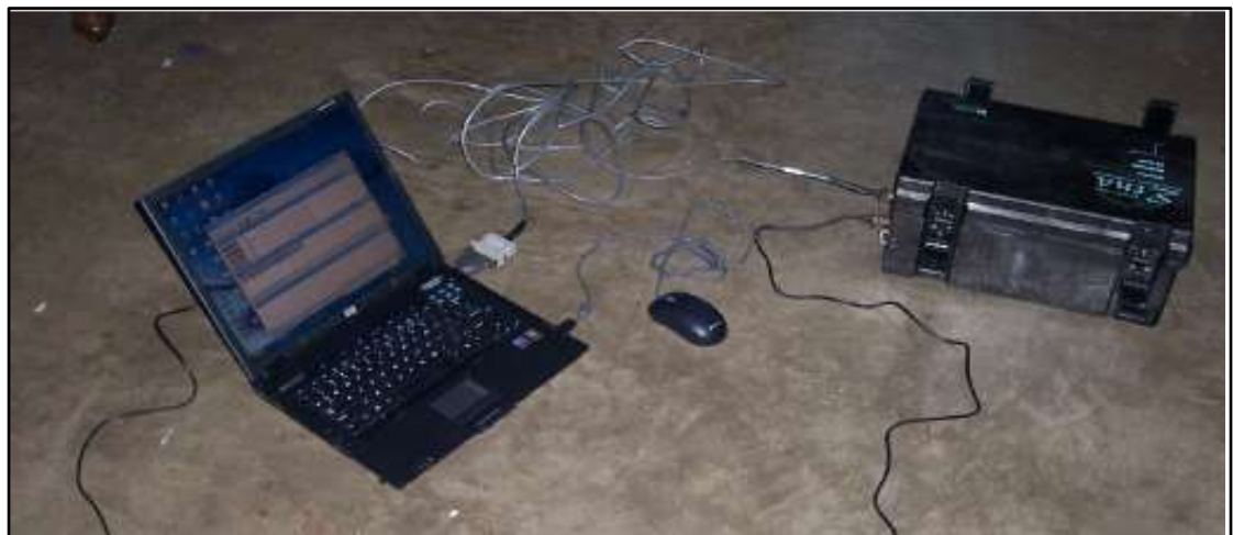
Figure 3.4: Obtaining the recorded data from accelerograph using laptop.
