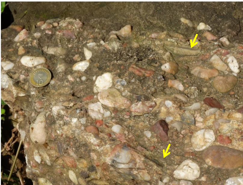
Figure: 3.13. Field Photograph of the matrix supported conglomerate facies (1B). Arrows indicate presences of mud clasts. The diameter of the coin is 2.5 cm.
