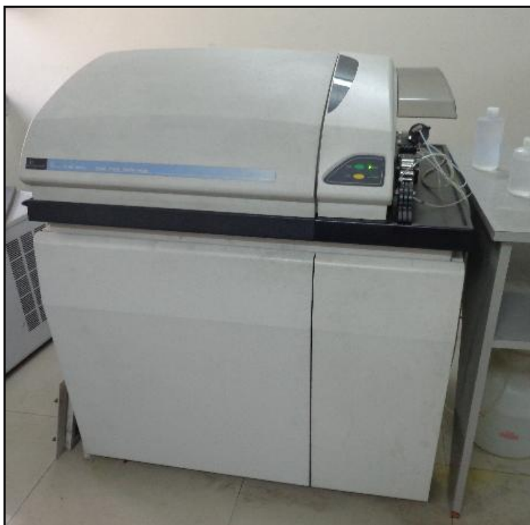
Figure 3.4 Photograph showing Inductively Coupled Plasma Mass Spectrometer (ICP-MS: Perkin Elmer, ELAN DRC-e) at the Institute Instrumentation Centre, IIT- Roorkee.
