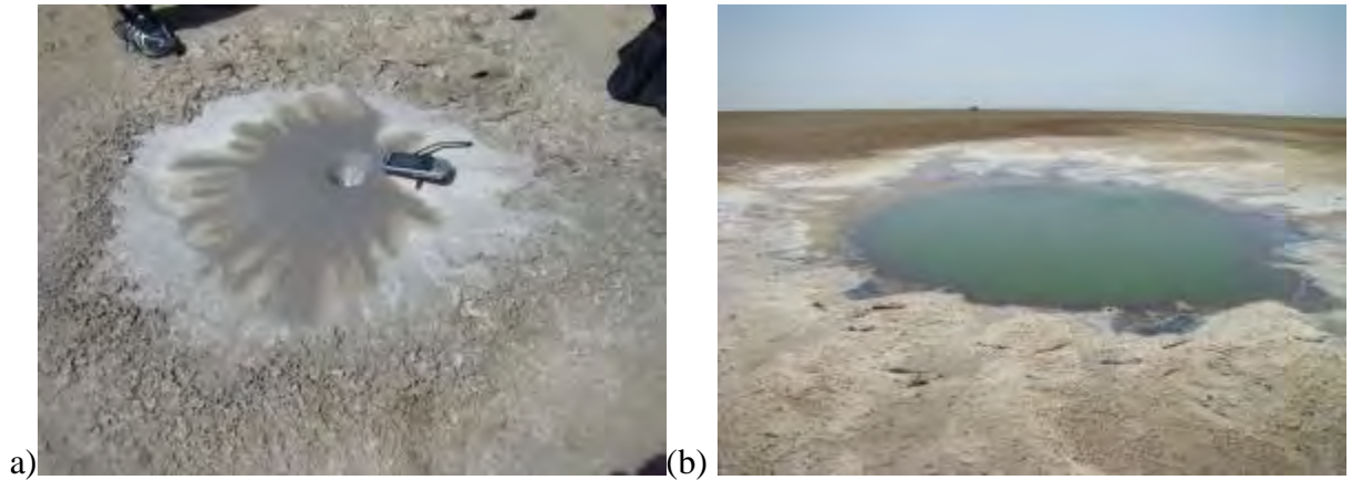
Figure 5.7: Liquefaction effect (a) Sand-blow liquefaction crater and (b) water pond near Dudhai village (figure 5.2) during May 2009 (courtesy: ISR 2010).
