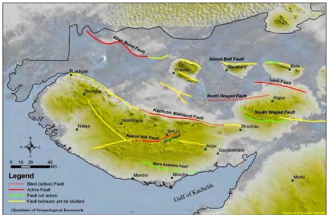
Figure 6.15: Active fault map of Kutch (ISR 2010).
