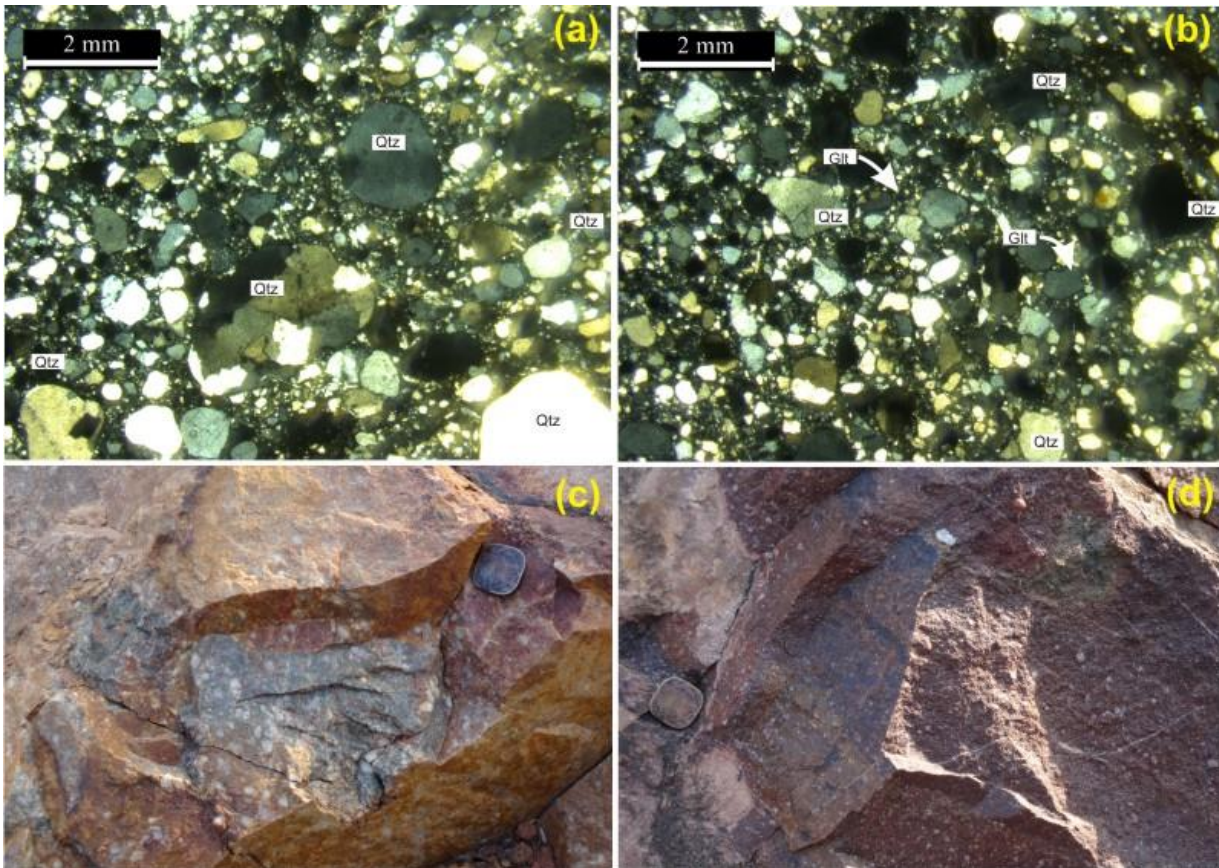
Figure 4.10: Photomicrographs (a&b) shows the rounded and multiple grains containing grains of quartz with their outcrop images of sandstone below in (c&d).
