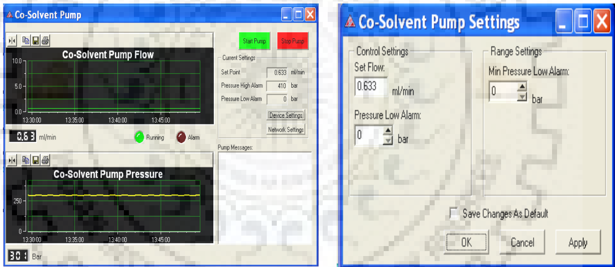
Fig. 3.9 Co-solvent pump setting in Process Suite software.
