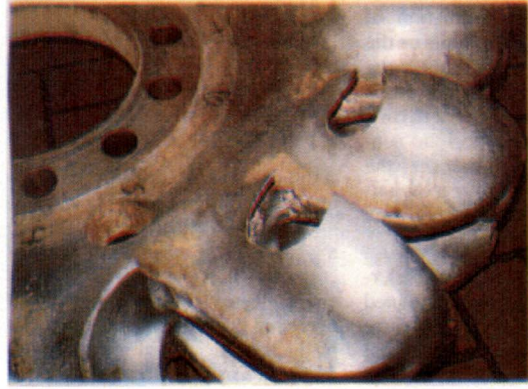
Fig. 1.33 A Pelton runner destroyed (P=10MW, H=410m) [24].
