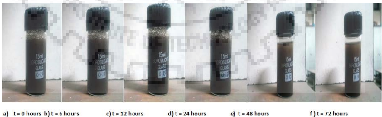
Figure 3.8 (b) : Photographic view of 0.05 % by volume of Copper Oxide nanoparticles in distilled water exhibiting settling of nanoparticles at different time intervals
