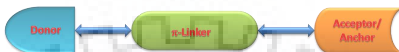
Figure 1.2 Pictorial representation of typical D- \pi -A configuration of organic sensitizers used in DSSCs.
