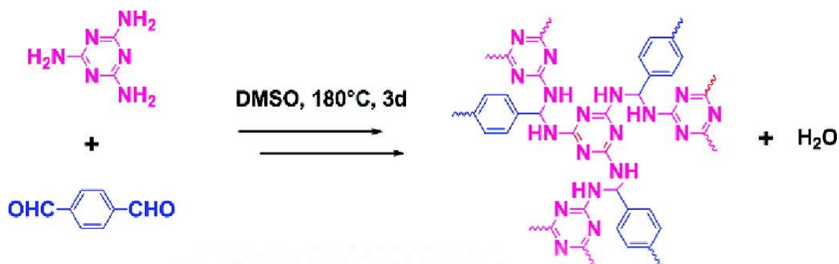
Figure 1.15: Synthesis of amorphous POP (SNW-1) by Schiff base condensation of terephthalaldehyde and melamine under catalyst-free condition. [Reprinted with permission from ref. 267 © 2009 ACS Publisher]
