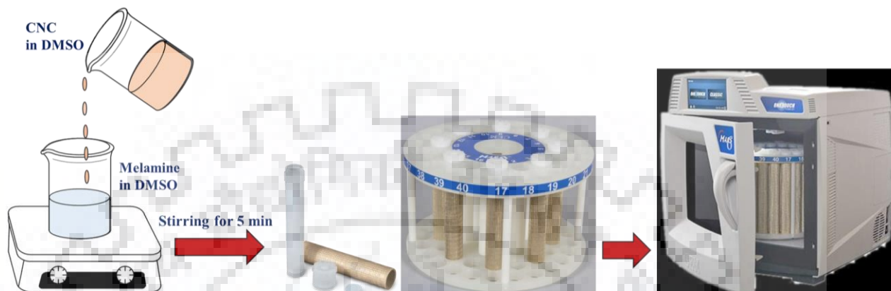
Figure 2.5. Procedure for the synthesis of NENPs using microwave-reactor assisted method.
