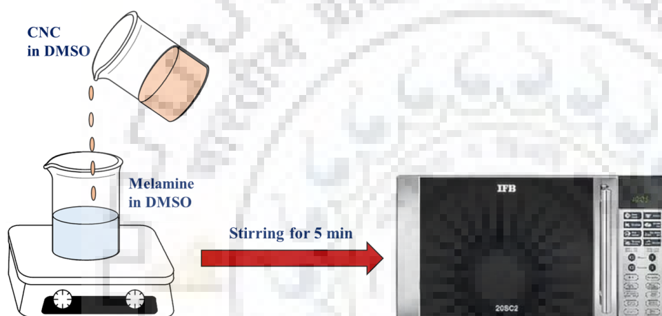
Figure 2.4. Procedure for the synthesis of NENP using domestic microwave oven.
