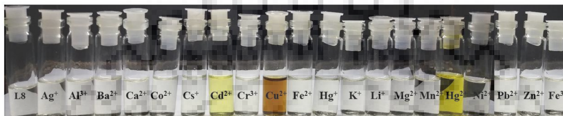
Figure 5.2. The colorimetric test of L8 with different metal ions in aqueous medium.
