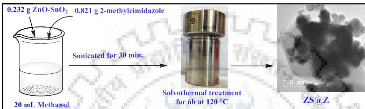
Scheme 6B.1. Schematic illustration of synthesis of ZS@Z.
